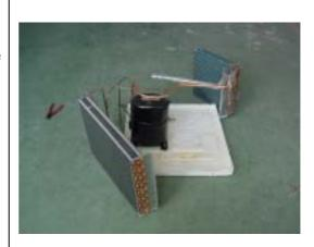
(17) Disconnect the piping and the compressor.
