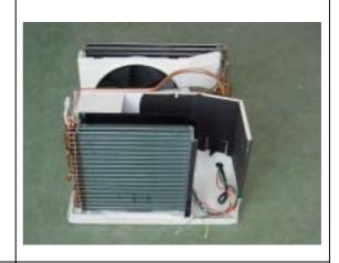
(8) Removal of evaporator assembly
