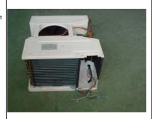
(5) Removal of front cover plate Unscrew the eight screws at the front cover plate and remove it.
