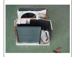
(7) Remove the bracing
