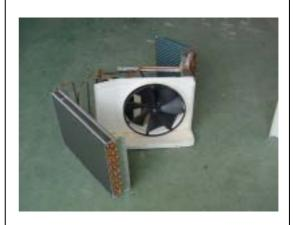
(14) Removal of propeller fan
