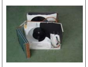
(10) Removal of centrifugal fan Unscrew the bolt at the centrifugal fan and remove it.
